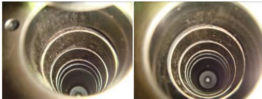
Plunger Block 內部磨損
