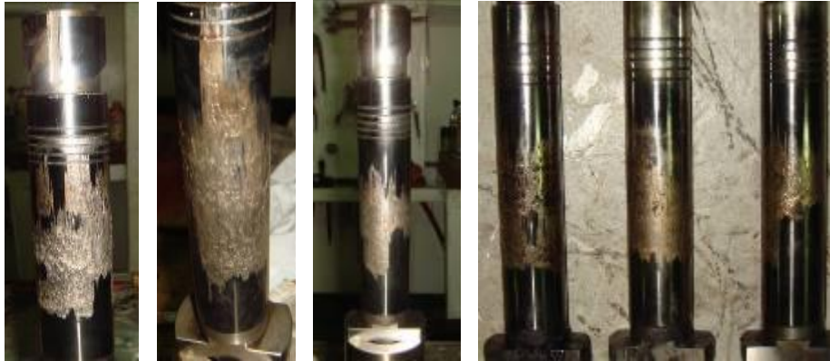
Plunger Block 內部磨損
